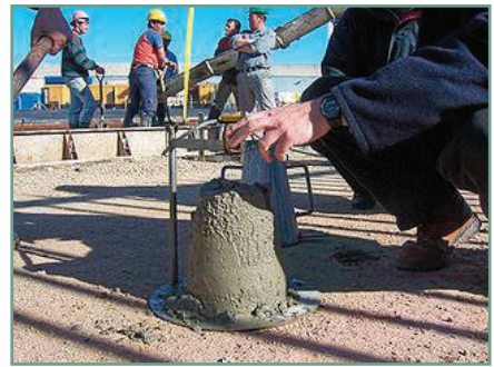
Figure 28: Measuring difference in height after removal of cone
