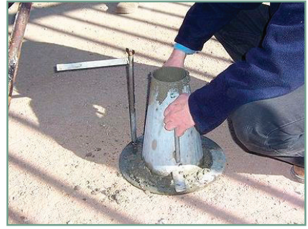
Figure 28: Measuring difference in height after removal of cone
