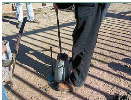
Figure 26: Tampering with rod in layers
