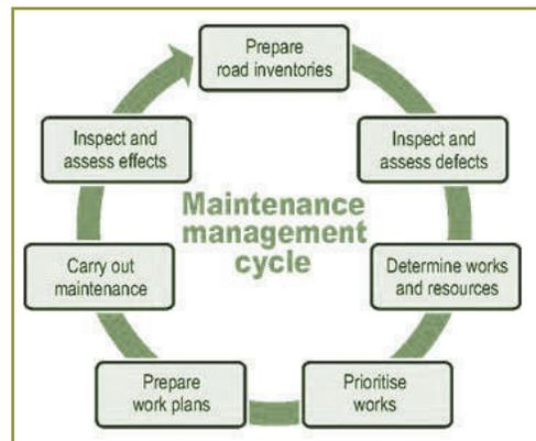
Figure 1 shows the maintenance management cycle with the various steps and their logical sequence necessary for achieving an effective maintenance management system.
